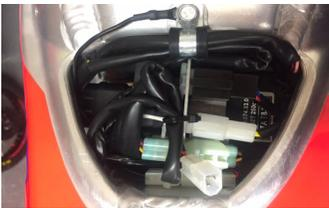
Separate all connectors and make sure they are pushed together correctly. Spray with electric spray. Also separate the CDI and spray with electric spray. **IMPORTANT.** Available from us.
